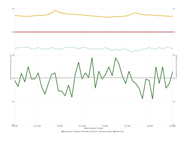
**Test Result: Below EPA Recommended Action Level**
